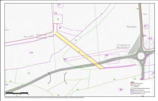
**Site 49** is a utility corridor associated with the Western Portal and Main Civils Compound elements of the Scheme. The utility corridor is shared to provide temporary and permanent water and power connections between the compound and the portal/tunnel support buildings.
